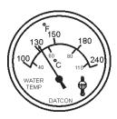
Figure 51. Coolant Temperature Gauge
